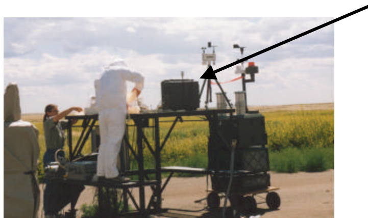
Figure 5 – 4WARN Sentry during field trials shown with referee equipment
