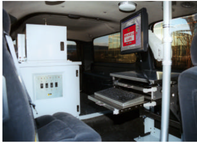
Figure 8 – Inside view of the 4WARN Urban showing the control console. The console can control a scalable network of detectors. Installation kits for other vehicles are also available.
